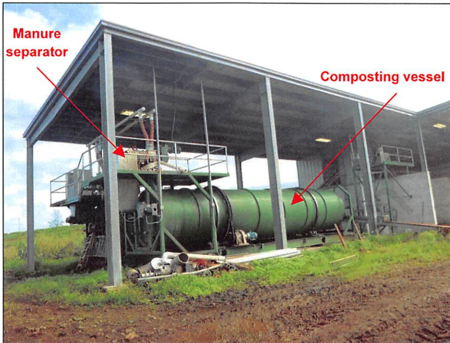
Photograph 17. View of the Facility's manure composting building which included two manure separator units, and two composting digester vessels. Photo by A. D'Angelo; 12/14/16.
